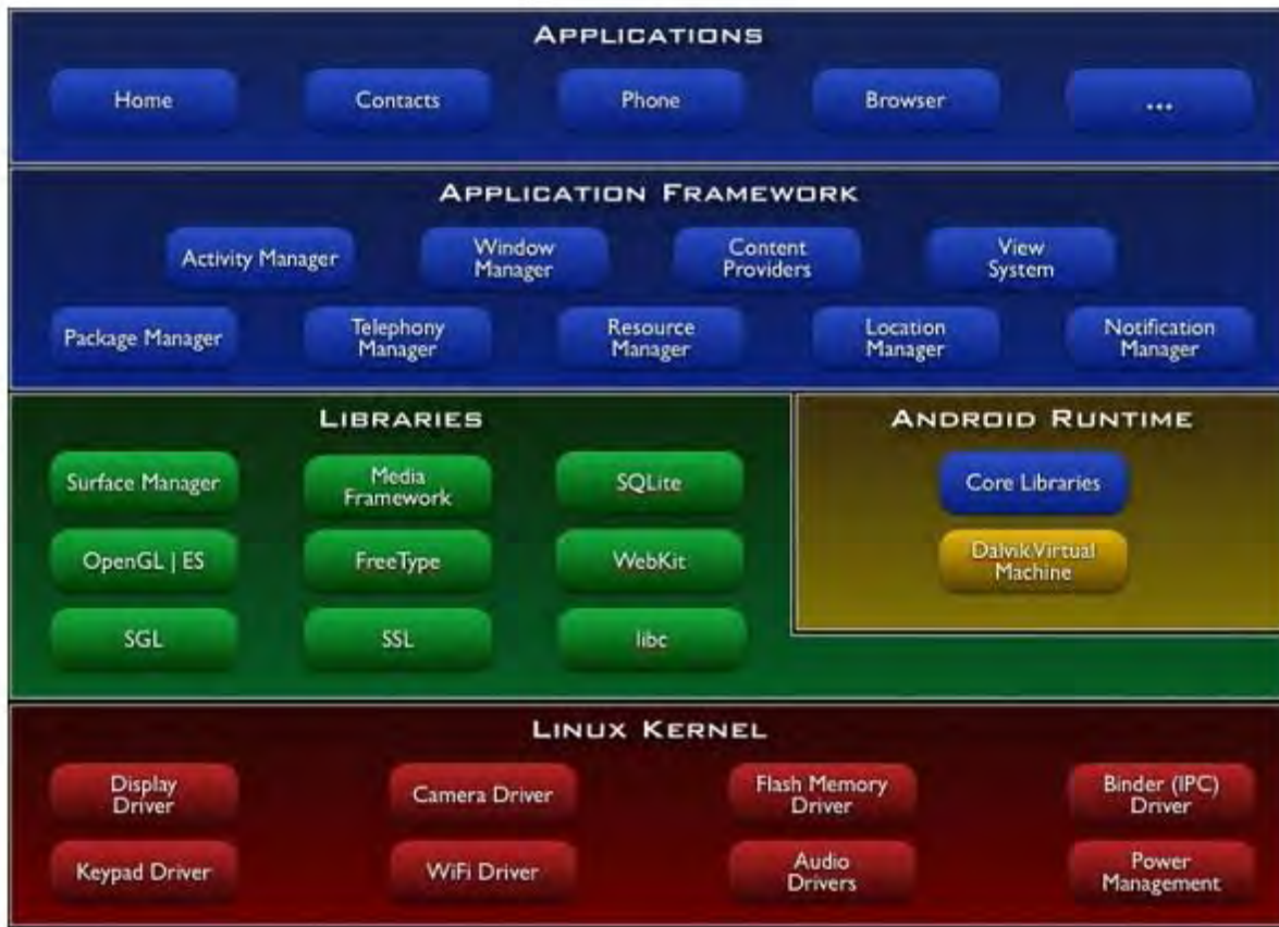
Figure 2-1 Android low level system architecture
